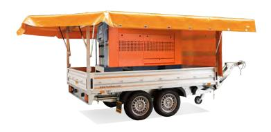
Device including stowage with weighing device and 4  ${\rm SF_6}$  cylinders on the B175R11L057 trailer
